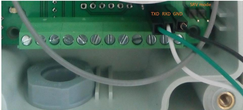
*Figure 2 UART & service mode pins in LPMDL-1101-2-reed*
